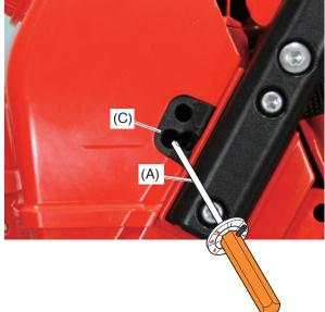
1. Start and warm engine for 1 minute alternating engine speed between WOT and idle every 5 seconds. Turn H mixture needle (C) anticlockwise until engine speed drops to approx. 12,000 r/min at WOT.
