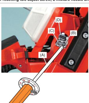
Tools Required: Small screwdriver with 2.5 mm blade, P/N G310-000050 electronic tachometer, P/N Y089-000090 D-shaped tool (A).
